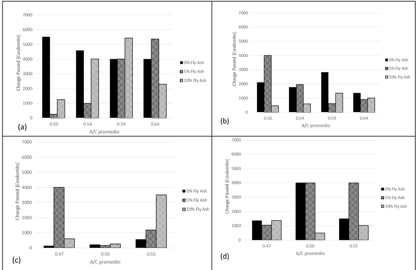
**Fig. 3.** (a) Charge Passed 14 days after casting for concrete samples (b) Charge Passed 28 days after casting for concrete samples (c) Charge Passed 14 days after casting for mortar samples (d) Charge Passed 28 days after casting for mortar samples
