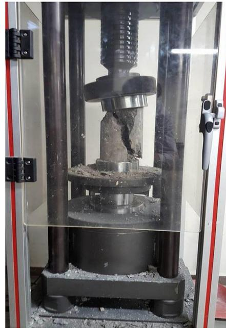
**Fig. 6.** General fracture pattern of the samples
